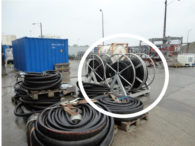
Figure 7 - 2 Hose Winders LHW 40/2-AL with hydraulic hoses for LSS 15m
