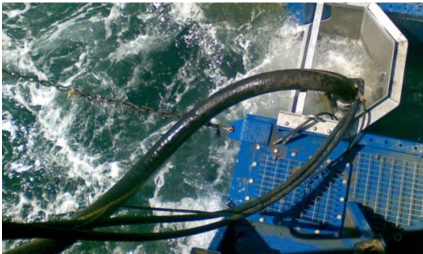
Figure 9 LSS 15 m, oil hose connected to weir skimmer module
