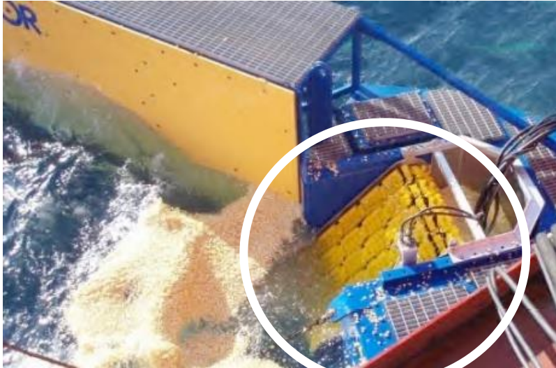
Figure 5 LAMOR Stiff Sweeping Arm Frame – brush skimmer module
