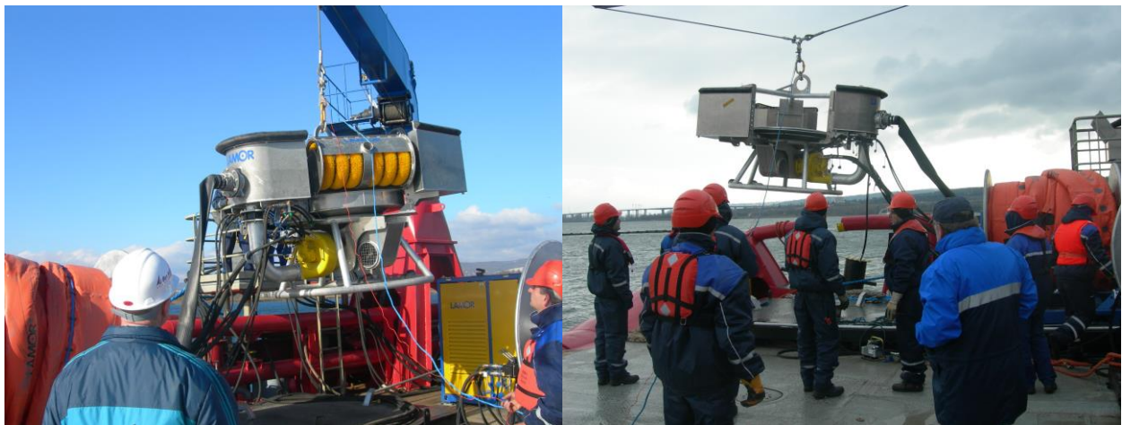
Figure 12 – Weir Skimmer LWS 1300 Mk II with brush and weir modules
