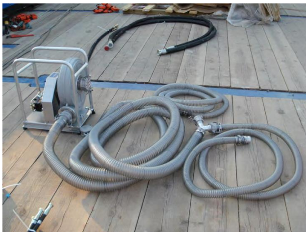
Figure 19 Hydraulic Air Blower HAB 200 and air hoses
