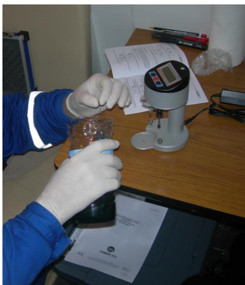
Figure 23 Mini-Lab for Oil Viscosity and Density
