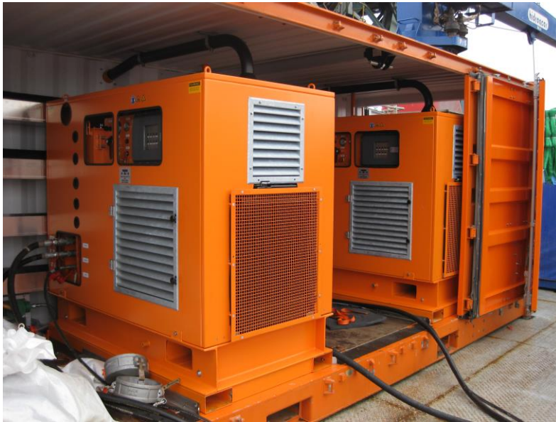
Figure 30 Vikoma weir boom power packs in container
