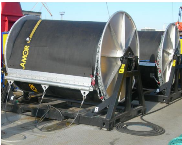
Figure 15 Oil Boom – Lamor Heavy Duty Boom (HDB) 2000
